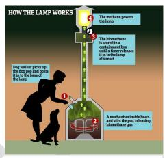
UKs first streetlamp powered by dog litter. Ten bags of litter power the light for 2 hours.
